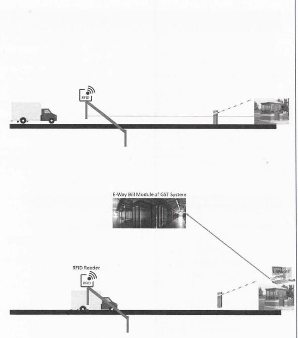
RFID Reader is connected to Facilitation Centre which Pulls records of e-Way Bill connected with the RC of Truck
